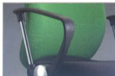
V1 - Venus Armrest Injection moulded reinforced polypropylene with chrome tubing and knob cover.
